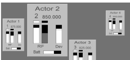
Fig. 2: Display of a scene configuration with four actors on the S-MCD Mikroport computer display
